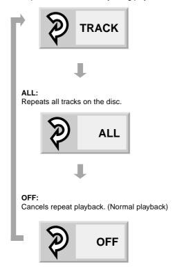
Repeat playback does not work for a Video CD with PBC function on. To turn off PBC, see "CHANGING SETUP VALUE" on page 38.
